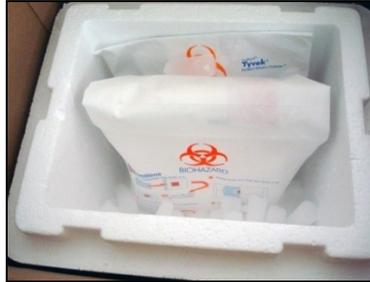
16. **FILL** the remaining space in the shipping carton with approximately 10 lbs of dry ice, ensuring ice surrounds the envelope(s) and reaches the top of the carton, as shown below:
